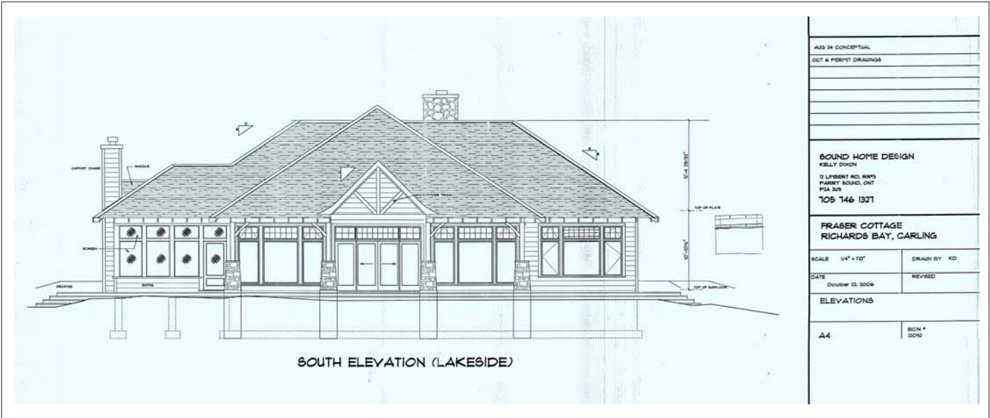
The 'Arts and Crafts' style exterior features dry stack limestone based cedar columns, 'rafter tail' porch overhangs, aluminum clad wooden windows, cedar decking and 'Gemthane' wood siding, all ensuring low maintenance.
